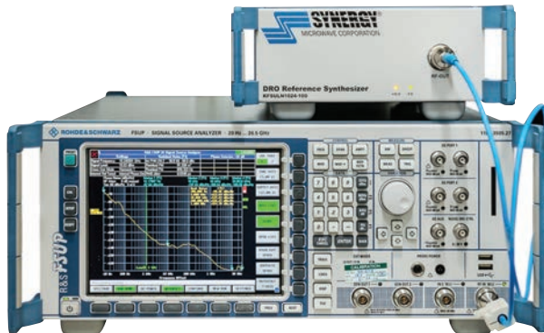
5 This measurement setup was used to test the DRO reference synthesizer.
