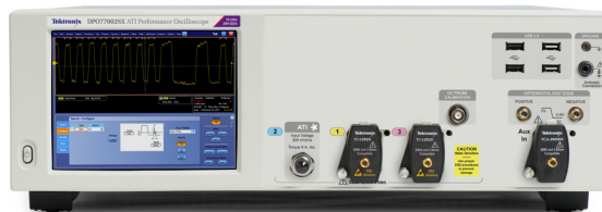
3. The model DPO70000SX 70-GHz real-time oscilloscope fits in a compact housing. (Photo courtesy of Tektronix)
