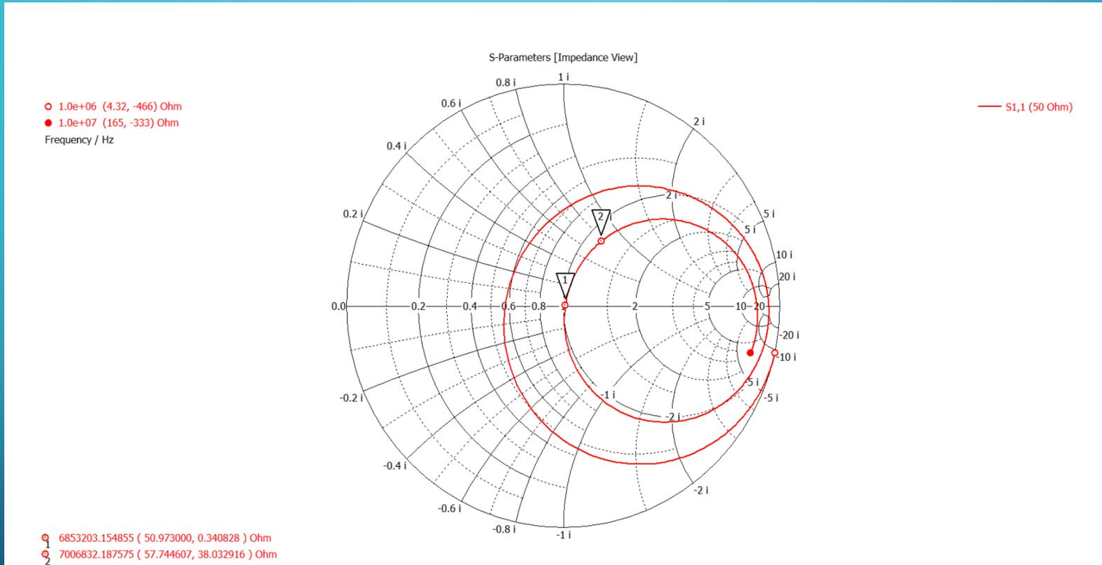
Fig. 19: Simulated Antenna Input Impedance
