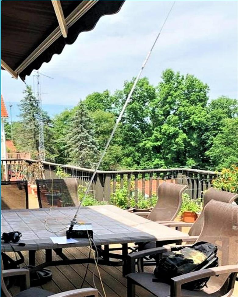
**Fig. 8: Military Manpack with a straight whip antenna**
