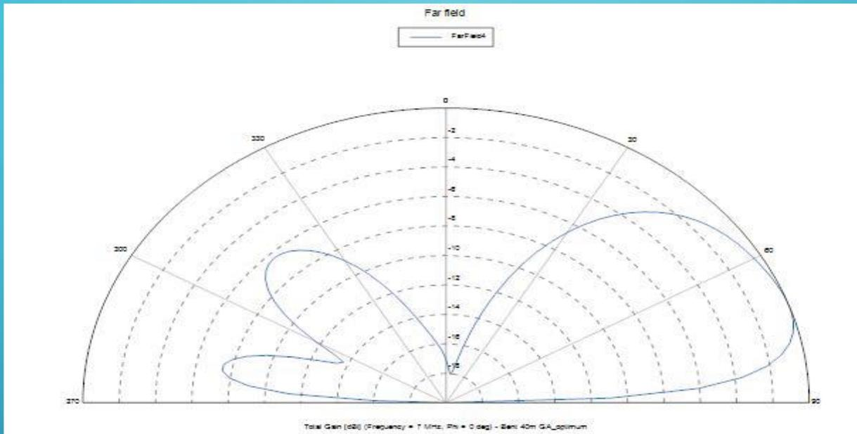
Figure 24: Elevation Pattern
