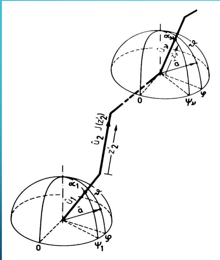
Fig. 11: 3-dimensional curvilinear monopole approximated by  $n$  straight line sections: designations
