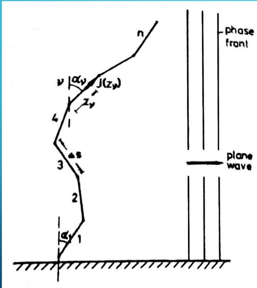
Fig. 9(b): Curved antenna split in numerous sections for analysis
