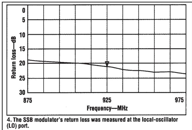
4. The SSB modulator's return loss was measured at the local-oscillator (LO) port.
