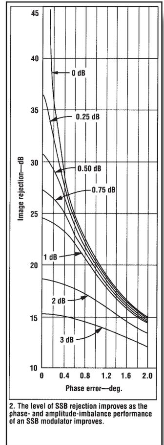
As an example, an SSB modulator is assumed to operate with +10-dBm LO drive with each modulating signal at -10 dBm and in phase quadrature to each other when applied to the modulating ports (MOD 1 and MOD 2). The result will be a modulated signal at -16 dBm, assuming 6-dB conversion loss. For 20-dB carrier rejection with respect to the desired modulated signal, the carrier must be at -36 dBm, which translates to LO-to-RF isolation of 46 dB.
