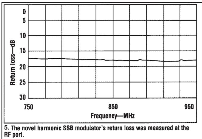
5. The novel harmonic SSB modulator's return loss was measured at the RF port.
