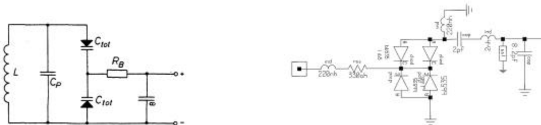
Figure 12 - Parallel-resonant circuit with two tuning diodes, on the left. To reduce the losses the better circuit uses two diodes in parallel on each leg. The shorted stub (SST) is a model element for a ceramic resonator.
